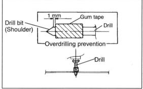
Drill the hole using a φ3-mm drill bit followed by a φ10-mm drill bit.
