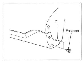
3. Using the front mud guard fasteners, install the front of the side air dam skirt.
