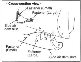
2. Align the side air dam skirt clips with the installation holes, inserting the 9 clips on the upper side first, then the 5 clips on the lower side.
