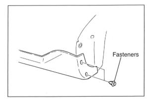
Align the side air dam skirt along installation positions, and temporarily reinsert the two front mudguard fasteners removed in "4. PART REMOVAL."
