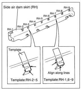
Align the two attachment areas on the template and affix it to the side air dam skirt as shown in the figure. (7 locations)
