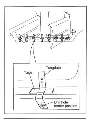
Leaving the template attached to the vehicle, remove the side air dam skirt.
