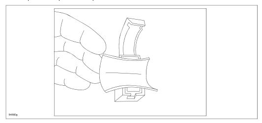
2. Install the protector clip on the emission harness by positioning it on the harness at the point shown (A), then squeeze the clip together until it snaps.
