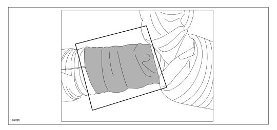
**TIP:** The work space for taping the harness is limited and may be difficult using a full roll of tape. Precutting 35 inches of tape, then wrapping it onto a 9mm or 10mm socket (A), allows easier application of the tape to the harness.
