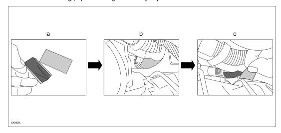
3. Using 35 inches of electrical tape, wrap the harness to completely cover the butyl taped area as shown.
